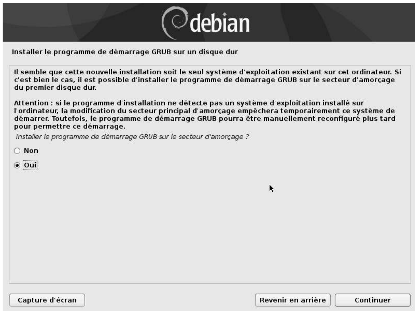
Installation : installation de GRUB
